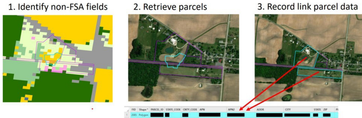
Figure 6: Example of overlapping agricultural fields with parcels to retrieve parcel landowner data (name, address, etc.). Once an agricultural field is identified (light blue polygon (1)), parcels overlapping that field are retrieved (purple polygons (2)) and the retrieved overlapping parcels (light blue polygons (3)) are record linked using name, address, and other tabular data.
