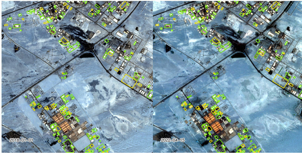
Figure 2: A 12.288 \times 12.288 \text{ km}^2 region in Dubai, UAE at (left) the beginning and (right) end of the study period. Construction sites beginning before 2018, but ending after are annotated in green. Construction sites beginning after 2018 are annotated in yellow.
